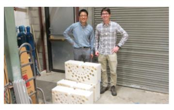
Nuclear physicists Tony Ahn and Zach Meisel stand on the dock at the Edwards Accelerator Lab and behind section of the polyethylene blocks used to slow down neutrons. The holes are where the detectors are placed.
