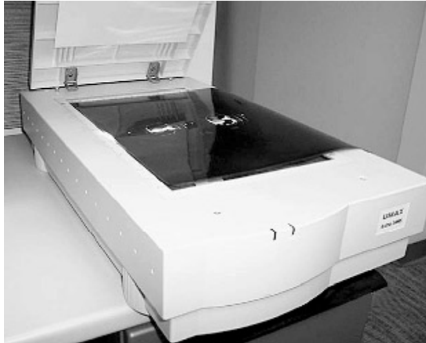
Figure 2: A flatbed scanner can be used to digitize a paper record. With a suitable backlight, X-ray films can also be digitized (photo credit: B. Harnett).
