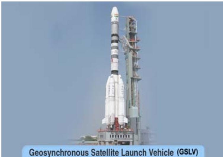
The 49 metre tall GSLV is a three stage vehicle. The first stage, GS1, comprises a core motor with 138 tonne of solid propellant and four strap-on motors each with 40 tonne of hypergolic liquid propellants (UH25 and N204). The second stage has 39 tonne of the same hypergolic liquid propellants. The third stage (GS3) is a cryogenic stage with 12.5 tonne of Liquid Oxygen and Liquid Hydrogen.
