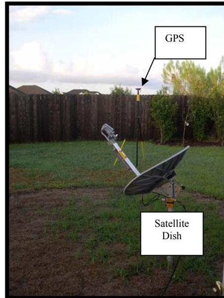
Figure 6.0 Broadband Internet Satellite Dish and GPS Antenna.
