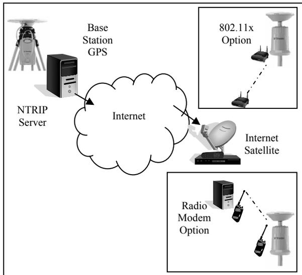
Figure 1.0 Space Based RTK configuration
