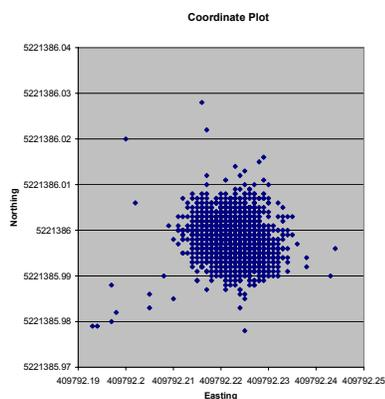
Figure 8.1 Coordinate Plot over two hours of time using SB-RTK
