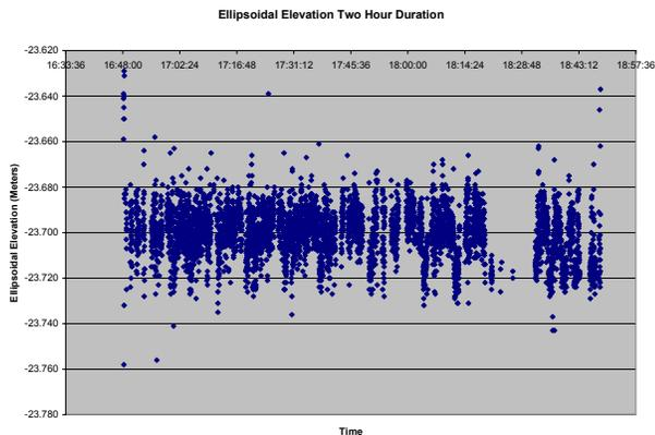
Figure 8.0 Elevation over two hours of time using SB-RTK
