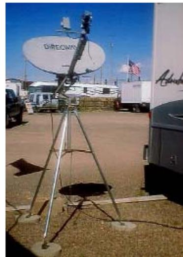
Figure 3.0 Directway broadband internet satellite antenna on tripod configuration.
