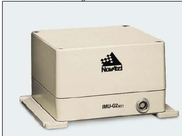
The HG1700 is connected to the OEM4-G2 via an Synchronous Data Link Control (SDLC) serial interface. Serial messages are transmitted at a 100 Hz rate from the IMU to the OEM4-G2. The first byte in each serial message triggers an interrupt serviced by a timing function tightly bound to the receiver's correlator chip. The time tag generated is accurate to 10 microseconds. The time tag is buffered while the rest of the 10 msec serial message is accumulated.
