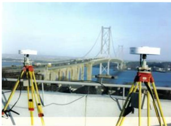
Figure 2, The two reference GPS receivers located adjacent to the Forth Road Bridge.
