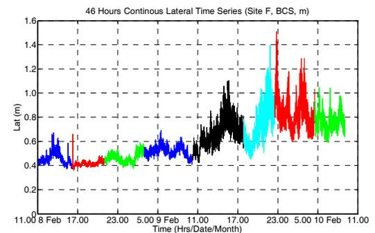
Figure 6, Lateral Deflections of Bridge site F over the 46 hour trial.
