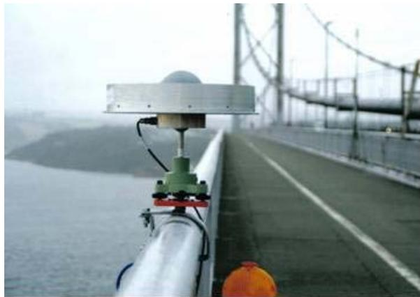
Figure 3, A Leica Choke Ring antenna located on the Bridge.
