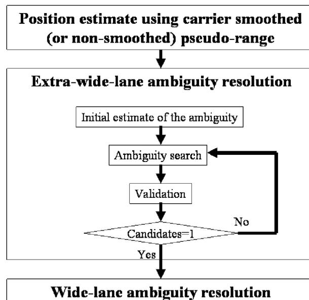
**Figure 1.** Flowchart of the RTK algorithm
