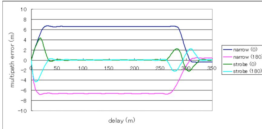
**Figure 3.** Multipath error envelopes for narrow and strobe correlator techniques
