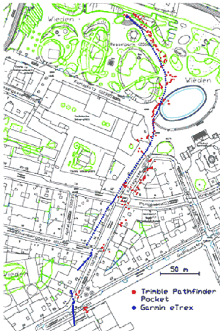
Fig. 1: GPS measurements for the pedestrian path from the underground station Karlsplatz to our office building of the Vienna University of Technology.
