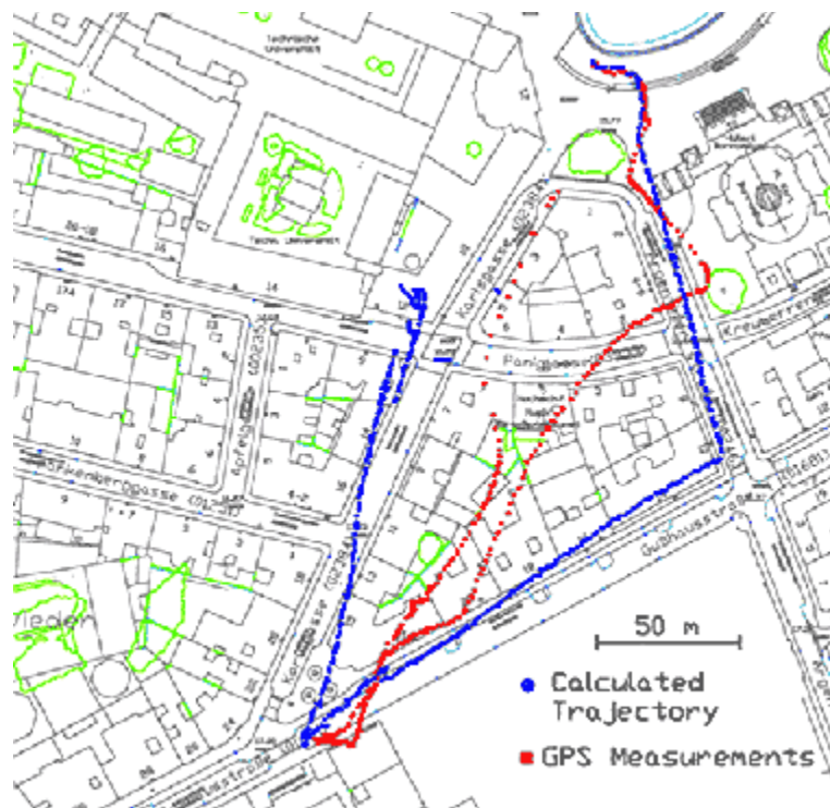
Fig. 5: Test measurements with the Dead Reckoning Module DRM III along a closed loop on narrow streets in the city Vienna
