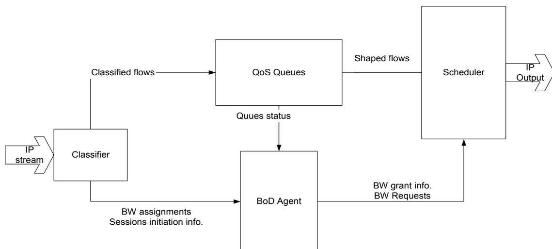
Figure 3: Simplified drawing of terminal BOD system
