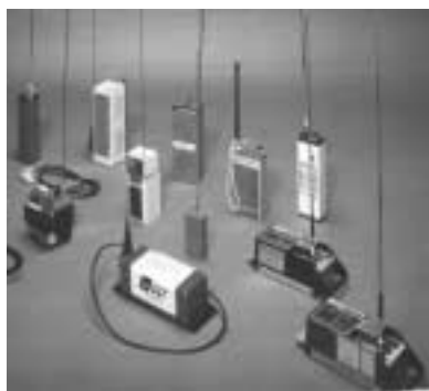
Figure 8: Typical 121.5 MHz ELTs used in aircraft
