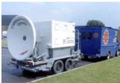
First SNG earth station in 1981 developed by CRC for CBC trials led to commercially built SNG trucks
