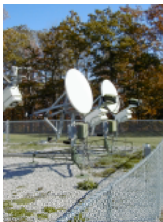
Figure 2 Rain Fade Compensation Experiment System
