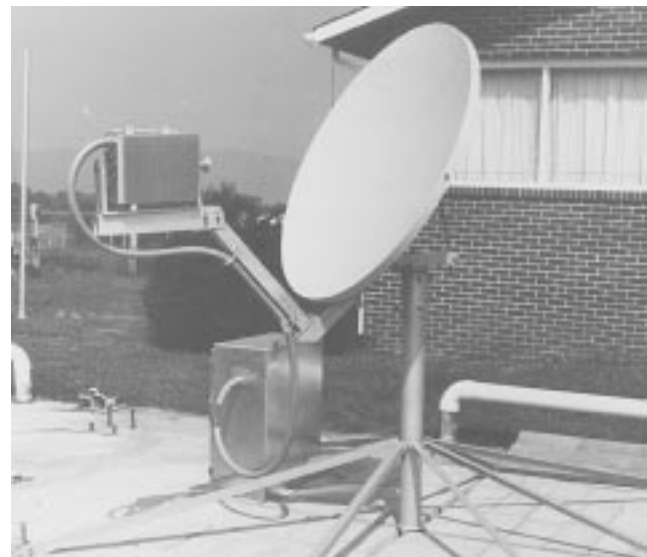
Fig. 5. ACTS 1.2-m receive-only propagation terminal.
